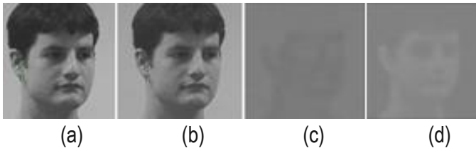
Figure 2. Channels in YCbCr format, (a) Original frame, (b) Y color channel, (c) Cb color channel, (d) Cr color channel
