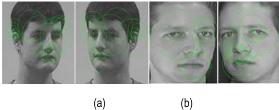
Figure 4. Example of Original Dataset Images Detected by SURF Feature Detector for both Left Image and Right Image. (a) Head Pose Dataset (b) ORL Dataset
