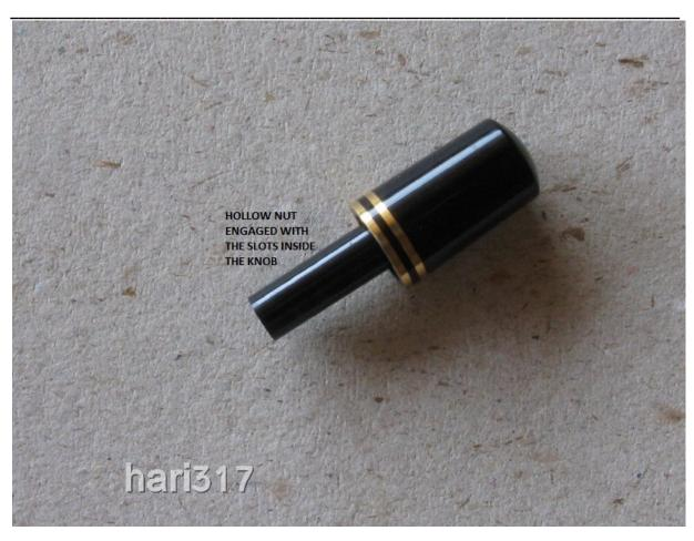
Reassembly: Engage the hollow nut into the filler knob and screw the knob onto the connector fully.
