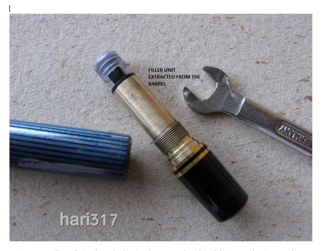
Maintenance will usually involve only cleaning the parts and applying lubricant to the piston seal. I use pure silicone grease.
